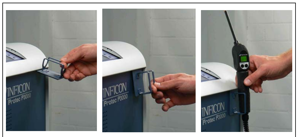
Fig. 8 Installation of sniffer line holder
