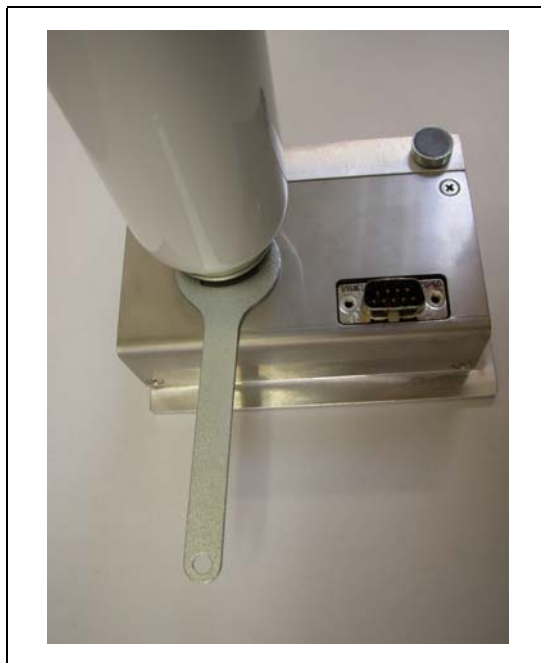
Fig. 87 Installing the gas reservoir
