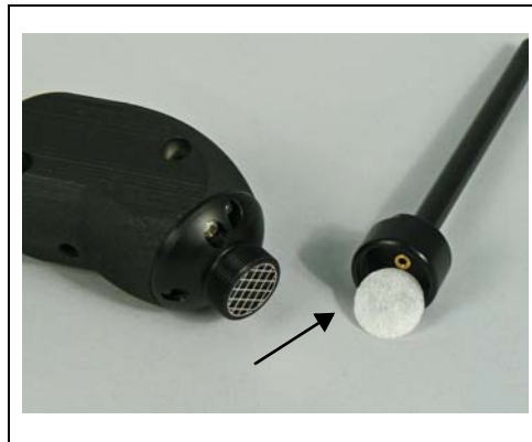
Fig. 79 Removed filter pad
