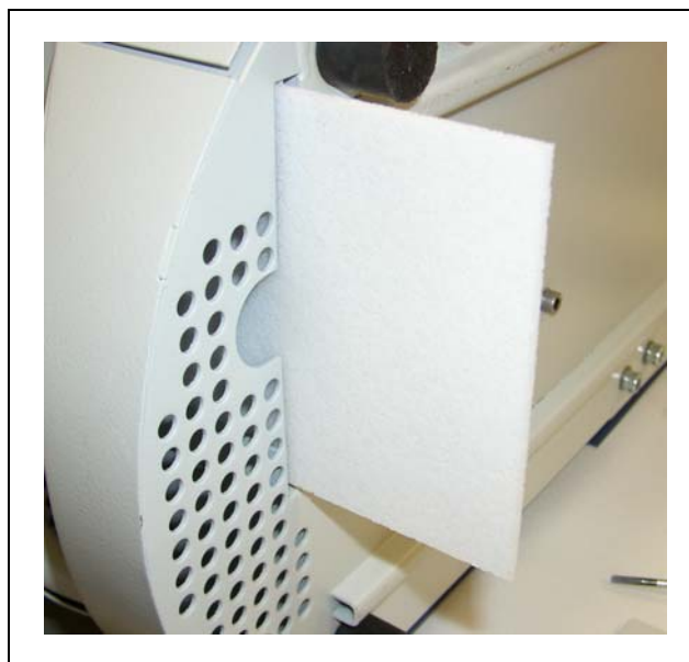
Fig. 71 Inserting the air filter
